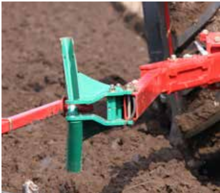
Packer arm connecting to the packer
